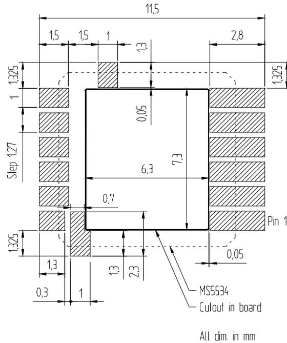
Pad layout for top side of MS5534B soldered onto printed circuit board
