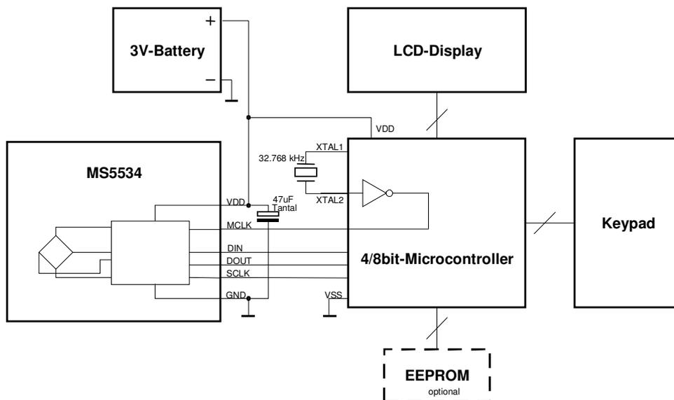
Figure 7: Demonstration of MS5534B in a mobile altimeter.
